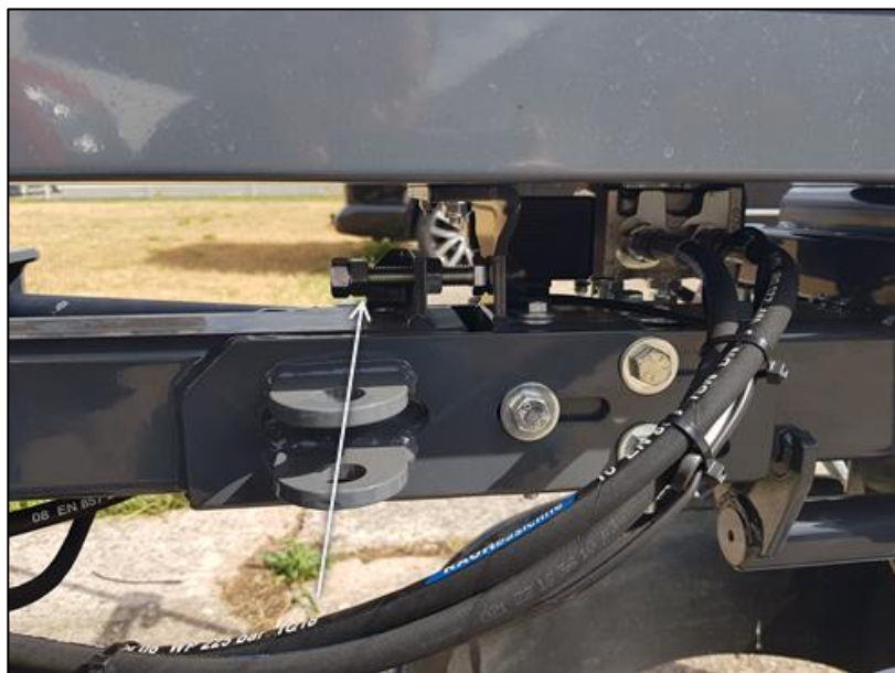
Fig. 29: Tension screw – belt drive
