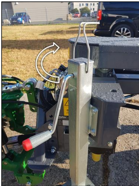
Fig. 21: Release the lock
