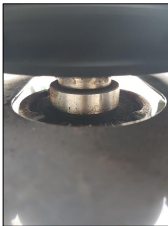
Fig. 7: Open the clamp ring on the pedestal bearing
