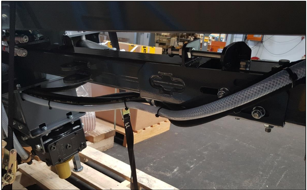
Fig. 12: Layout of the water hose
