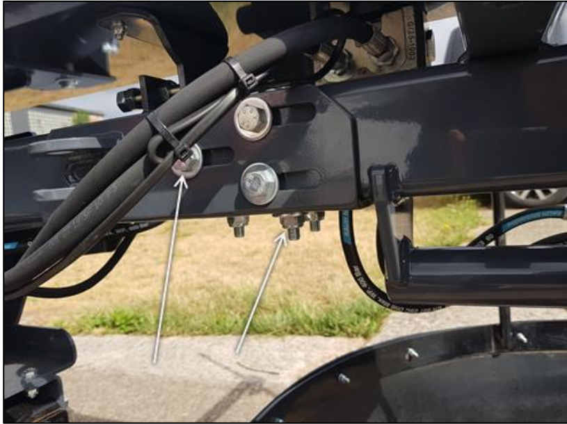
Fig. 27: Fastening screws – arm
