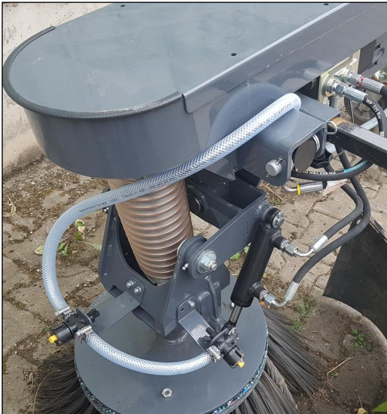
Fig. 11: Placement of the spray nozzles
