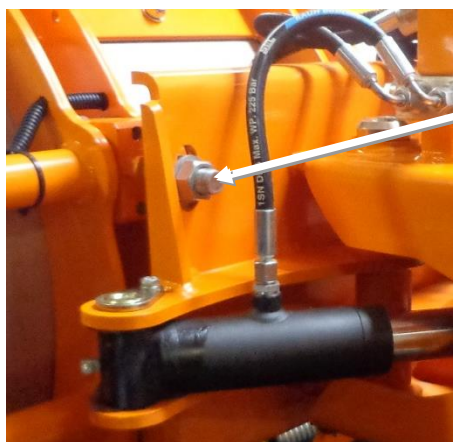
Fig. 8: Adjust the length of contact angle - set screw
