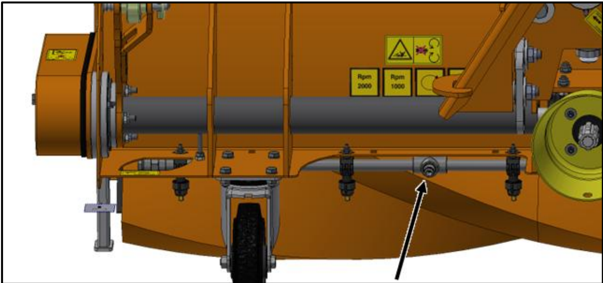
Fig. 56: Operation of water sprinkler
