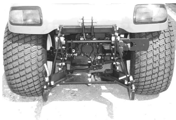
Fig. 12: Mounting the strut rods
