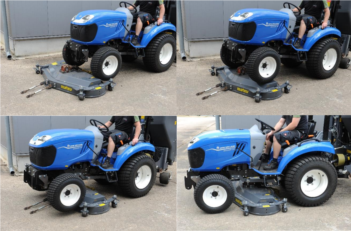
Figure 27 : Drive over mower
