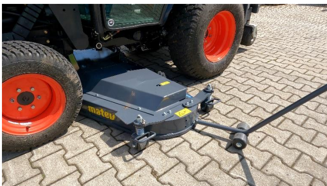
Figure 29 : Push the mower sideways under the tractor
