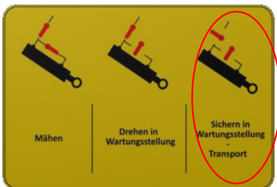
Fig. 36: The shut-off valves "Secure in maintenance position"
