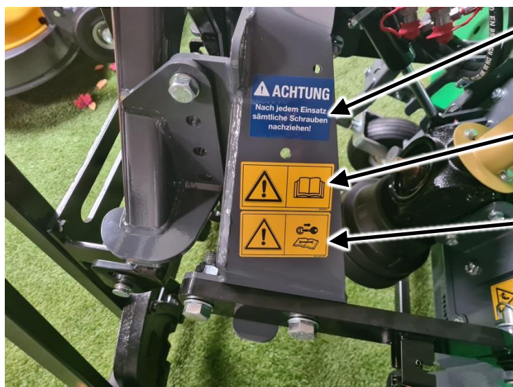
Fig. 11: Warning sign on the right attachment bracket
