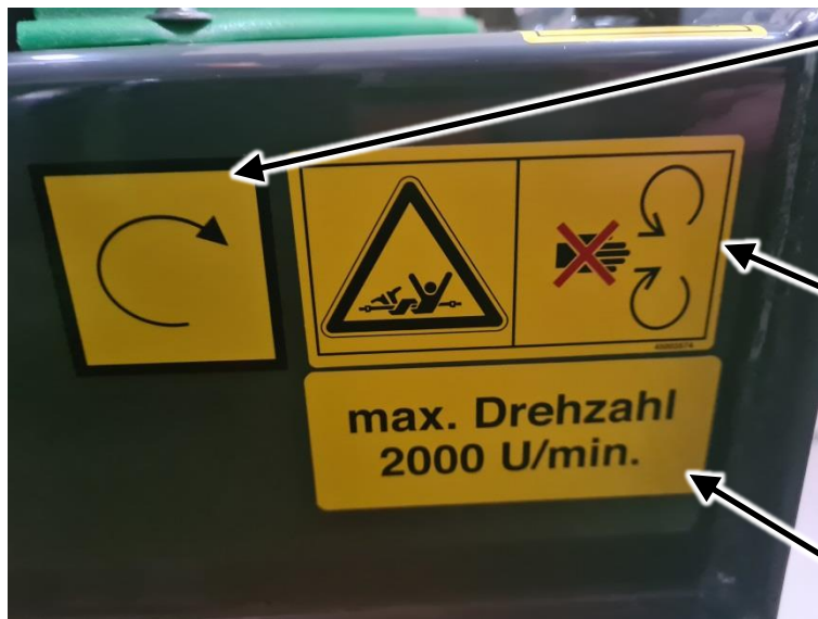
Fig. 14: Warning sign on the basic deck (right side discharge rear)
