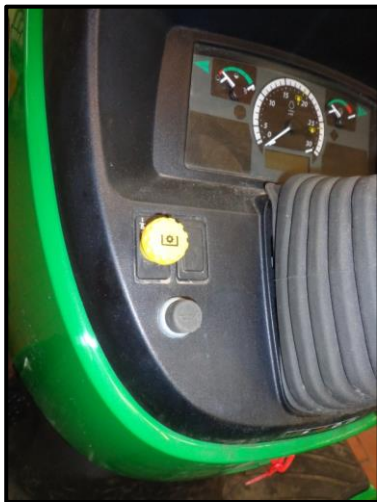
Fig. 12: PTO shaft switch (tractor without cab)
