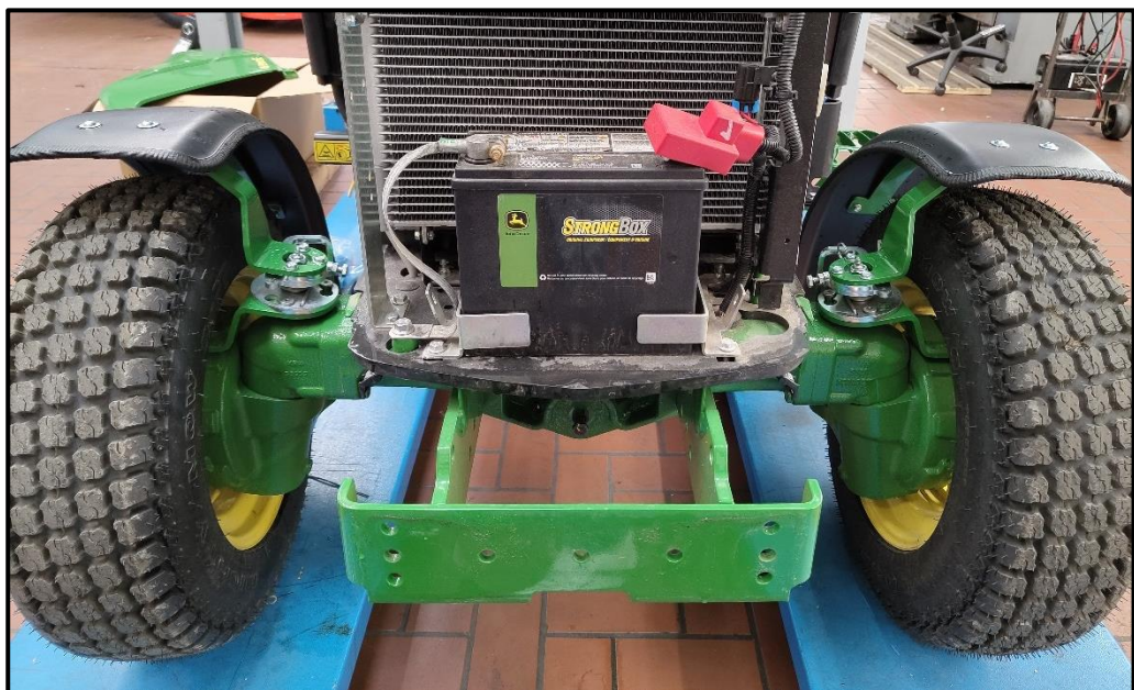
Fig. 1: Battery with bracket
