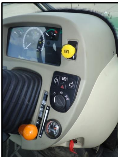
Fig. 13: PTO shaft switch (tractor with cab)
