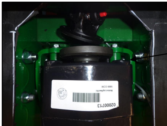
Fig. 7: Installation of the engine PTO shaft on the front linkage
