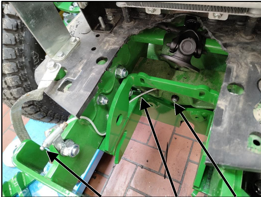
Fig. 5: Front axle Grease nipple Extension Screw
