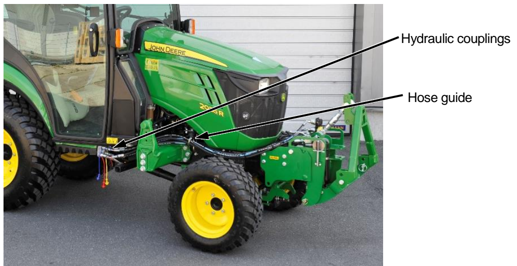
Fig. 6: Front power system hooked in
